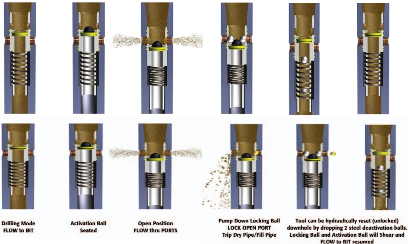
Activating and de-activating of the PBL tool is shown. (Images courtesy of Downhole Devices LLC)
