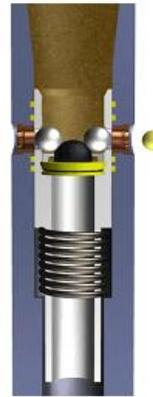
Tool can be hydraulically reset (unlocked) downhole by dropping 2 steel deactivation balls. Locking Ball and Activation Ball will shear and FLOW to BIT resumed.
