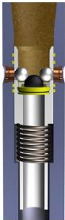
De-Activation Balls Dropped PRESSURE UP
